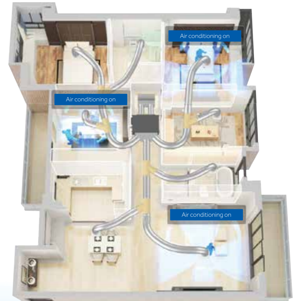
With SmartZone installed, air conditioning is switched on for only the three occupied rooms.
