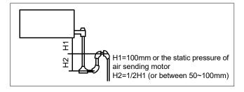
Taking the ADH\*\*H serials as an example, the installation of the drain pipe is the following.
